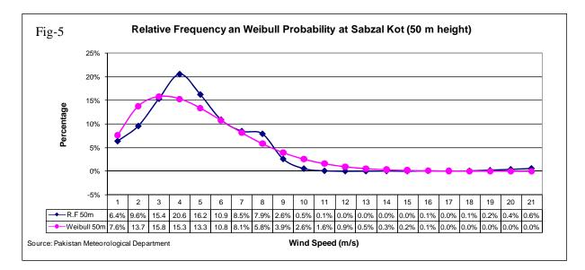
The Weibull parameters for four different heights 20 meters, 30 meters, 50 meters and 80 meters are given in Table-2 along with other key results of analysis.
