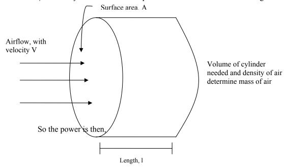
$$P = \frac{1}{2} \frac{dm}{dt} V^2 = \frac{1}{2} \varphi AVT / t V^2$$
