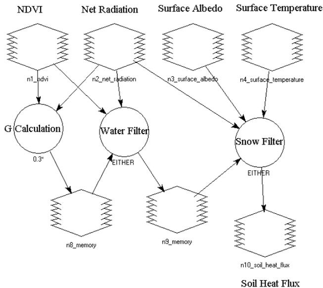
Figure 3: Model for Soil Heat Flux
