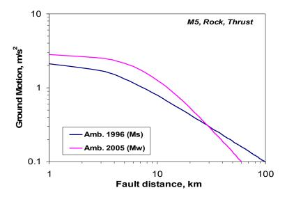
Figure 6.1.Comparison of predicted PGA using the empirical ground motion prediction equations by Ambraseys *et al.* (1996) and Ambraseys *et al.* (2005) for magnitude M 5.0.
