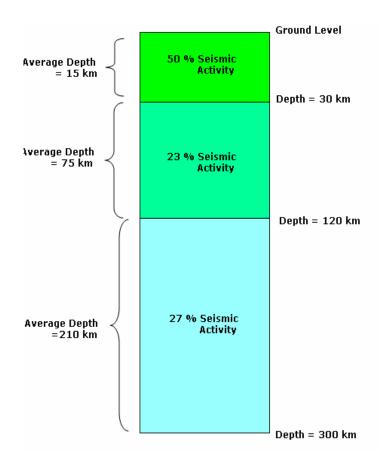
Figure 6.5.Representation of the seismic activity with respect to depth. The hypocentres of almost 50% of earthquakes in the Hindu Kush region and the northern areas of Pakistan lie within a range of 0 to 30 km.
