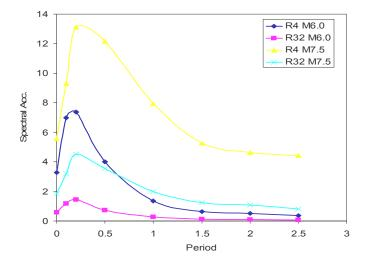
Figure 6.3.Spectral acceleration predictions for two magnitudes (6.0 and 7.5) and two distances (4 and 32 km) from Ambraseys *et al.* (2005).
