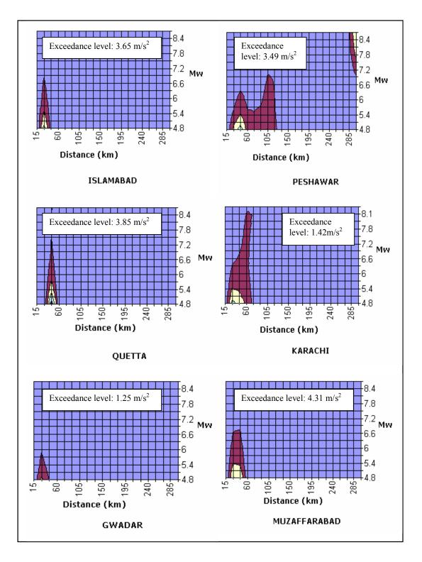
Figure 8.7. Deaggregation results for different cities at Peak Ground Acceleration.
