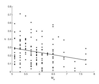
Figure 6.4.Observed dependence of  $\sigma$  on  $M_w$  using the binned data for PGA. The fitted line has the equation:  $\sigma = 0.5774 - 0.0561 \cdot M_w$  (Ambraseys *et al.*, 2005).
