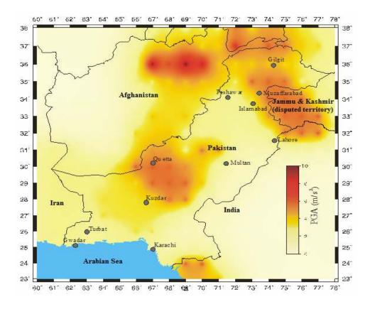
Figure 8.4. Seismic hazard map of Pakistan prepared for PGA for 500 years return period.
