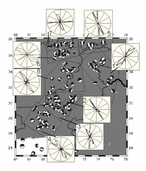
Figure 5.6.Focal mechanisms from the Harvard CMT solutions between 1977 and 2006. Inset are aggregated directions of maximum horizontal compression in the crust as derived from the focal mechanisms following the WSM recommendations (http://www-wsm.physik.uni-karlsruhe.de).
