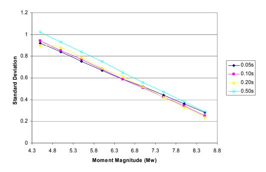
Figure 6.6.0bserved dependence of  $\sigma$  (standard deviation) on Mw using the data for PGA values.
