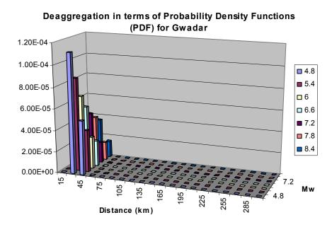
Figure 8.12. Probability Density Function (PDF) of Peak Ground Acceleration (PGA) for ground motion level at 5.75 m/s<sup>2</sup> for Gwadar.
